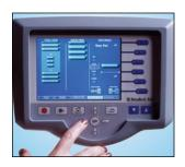
1. With the easy-touse control panel, the operator selects the number of tubes, their thickness and length.
