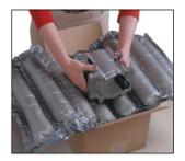
3. The operator centres the product on the tubes, setting both into the carton.
